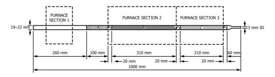
A = clear fused quartz section (optional when a translucent quartz tube is used)
