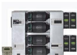
Each **FP4** is designed for 120/240 VAC single-phase output. Each power panel includes four inverter/chargers, four FM80 charge controllers, FlexNetDC, AC and DC wiring boxes, a MATE3, HUB10, and an AC/DC Surge Protector, X-240 transformer (not on FXR systems), inverter and controller breakers with GFDI, and an AC Input-Output-Bypass Assembly. Dimensions are 59"W x 46"H x 13"D. Weight is 520 lbs.
