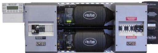
Each **FP2** is designed for 120/240 VAC single-phase output. Each power panel includes two inverter/chargers, two FM80 charge controllers, FlexNetDC, AC and DC wiring boxes, a MATE3, HUB10, and an AC/DC Surge Protector, X-240 transformer (not on FXR systems), inverter and controller breakers with GFDI, and an AC Input-Output-Bypass Assembly. Dimensions are 59"W x 21"H x 13"D. Weight is 260 lbs.
