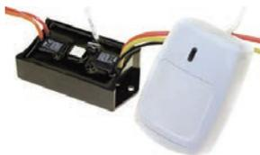
The fully-waterproof PVLC series charge and lighting controllers can be used with 12 or 24 VDC systems and are well suited for operating area lighting or signage. MD-designated controllers have a motion sensor to activate the light or load when motion is sensed. Controllers with and without motion detectors are available in 15 A and 40 A versions.
