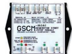
The GSCM-mini generator start controllers are optimized for use with OutBack Power and other inverters and charge controllers that have a 12 VDC output from their programmable AUX relay. They support three types of three-wire generator control: momentary, maintained, or ignition. They have a fixed crank time and over and under frequency shutdown. 2-year limited warranty.
