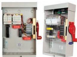
The MidNite **DLTL** disconnect combiners have both dual-string fusing and dual-channel output. These work for inverters with ungrounded conductors and dual-MPPT input channels which are becoming common. Both the positive and negative legs are fused, and the fuse holders are included. They are also available with the Rapid-Shutdown PSB circuit board installed.
