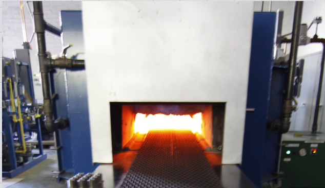
The connectors enter the furnace on a conveyor belt and a gas-tight hermetic seal is formed around all contacts, and between the glass seal and the connector shell, when the vitreous glass is melted in the furnace and then cooled under controlled conditions.
