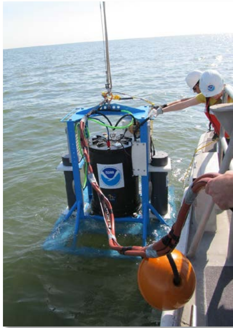
Image 4. In 2016, scientists from NOAA and the University of Michigan deployed ESPniagara for the first time in western Lake Erie. Scientists often refer to ESPs as “labs in a can” due to the technology’s ability to perform multiple, ongoing experiments in the field and provide daily bloom and toxicity information to researchers in a lab. The ESPniagara sensors provide data that complements other information gleaned by field monitoring through private enterprises and municipalities (Photo credit: NOAA/OAR/GLERL).
