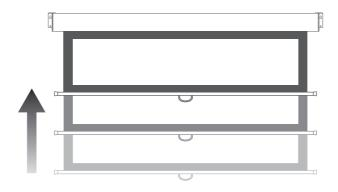
Pull down the screen and hold for 3 seconds, then release. The screen will stay at the desired position.
