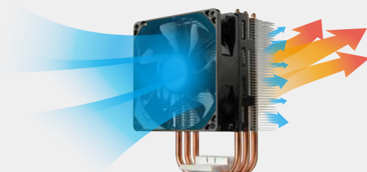
Others - Cooling air leaks from sides
