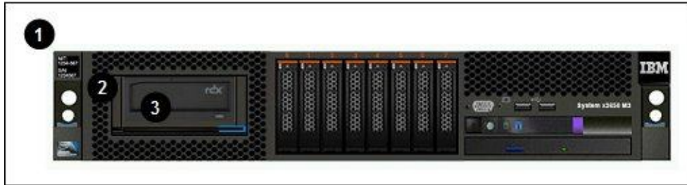
Figure 5. The IBM RDX Internal USB 3.0 Dock installed in an x3650 M3 server
