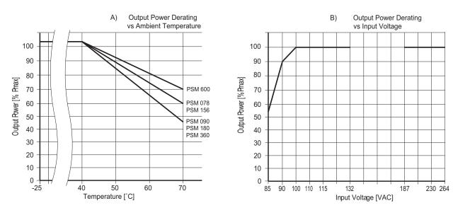
Note: Unless otherwise stated, all specifications are valid at nominal input voltage, full load and +25°C after warmup time.
