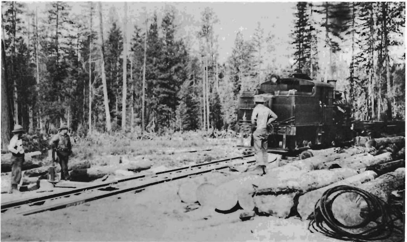
Heisler No. 102 pulling empty log cars backs into a siding at a reload on the "C" line in 1928.
