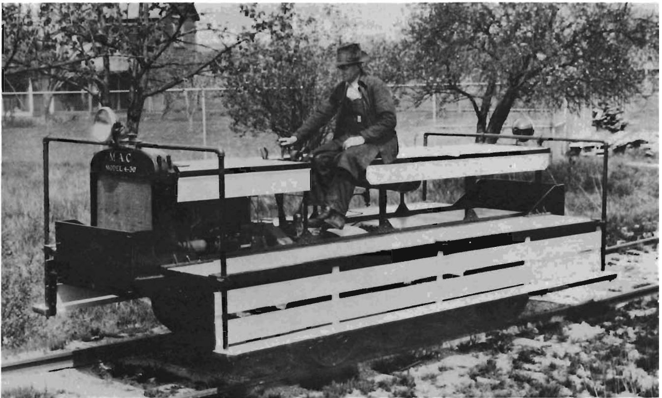
Builders photo of the Biles-Coleman Lumber Company "M. A. C. 4-30" speeder built by the Skagit Steel and Iron Works in February 1929. In this photo the speeder was equipped temporarily with standard gauge width axles for tests at the factory.
