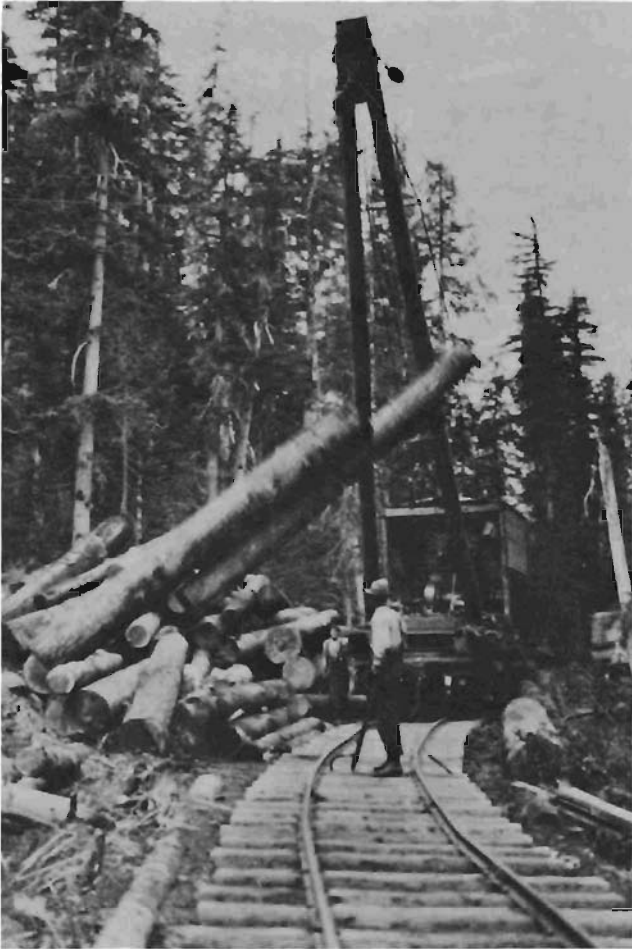
H. A. Peterson D. M. Co. slideback log loader skidding logs cut along the railroad right-of-way to trackside, July 1929.
