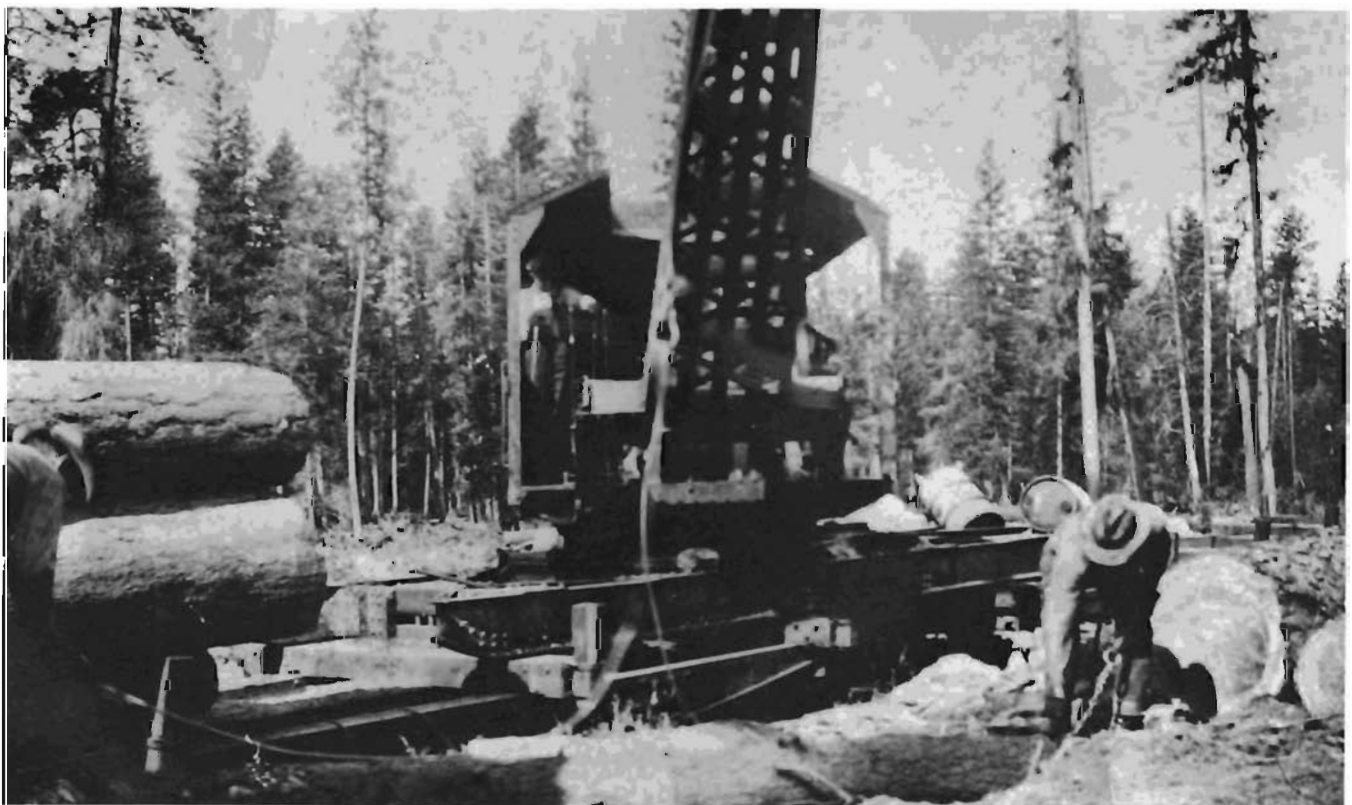
Hook tenders attach loading cables to the next log to be hoisted onto log car No. 109.
