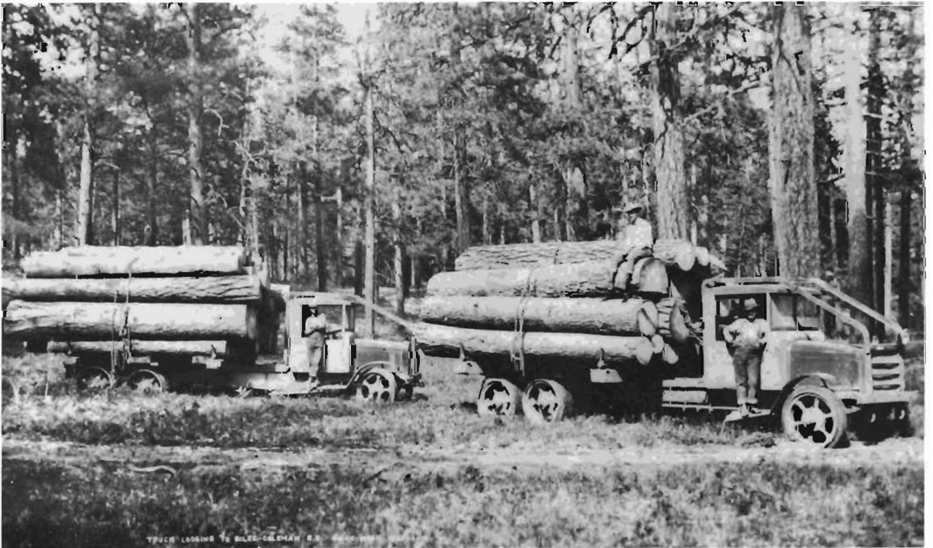
Ladd Photo from E. R. Aston Moreland solid tire log trucks carried logs over 5 to 6 mile runs to the narrow gauge. Photo taken near Camp 5 with Emmitt Aston sitting on top of the first loaded truck, 1927.
