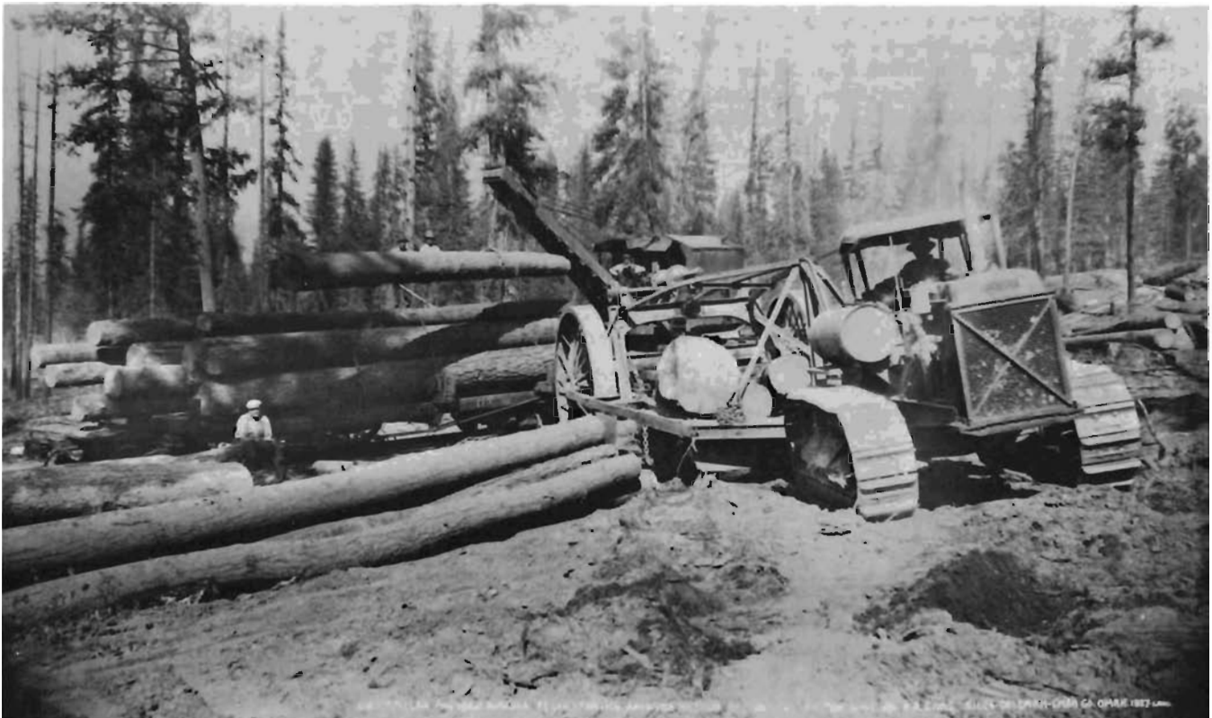
Caterpillar tractor, hydraulic lift high wheels, log car No. 119, and the slideback log loader highlight this 1927 Ladd Photo. E. R. Aston
