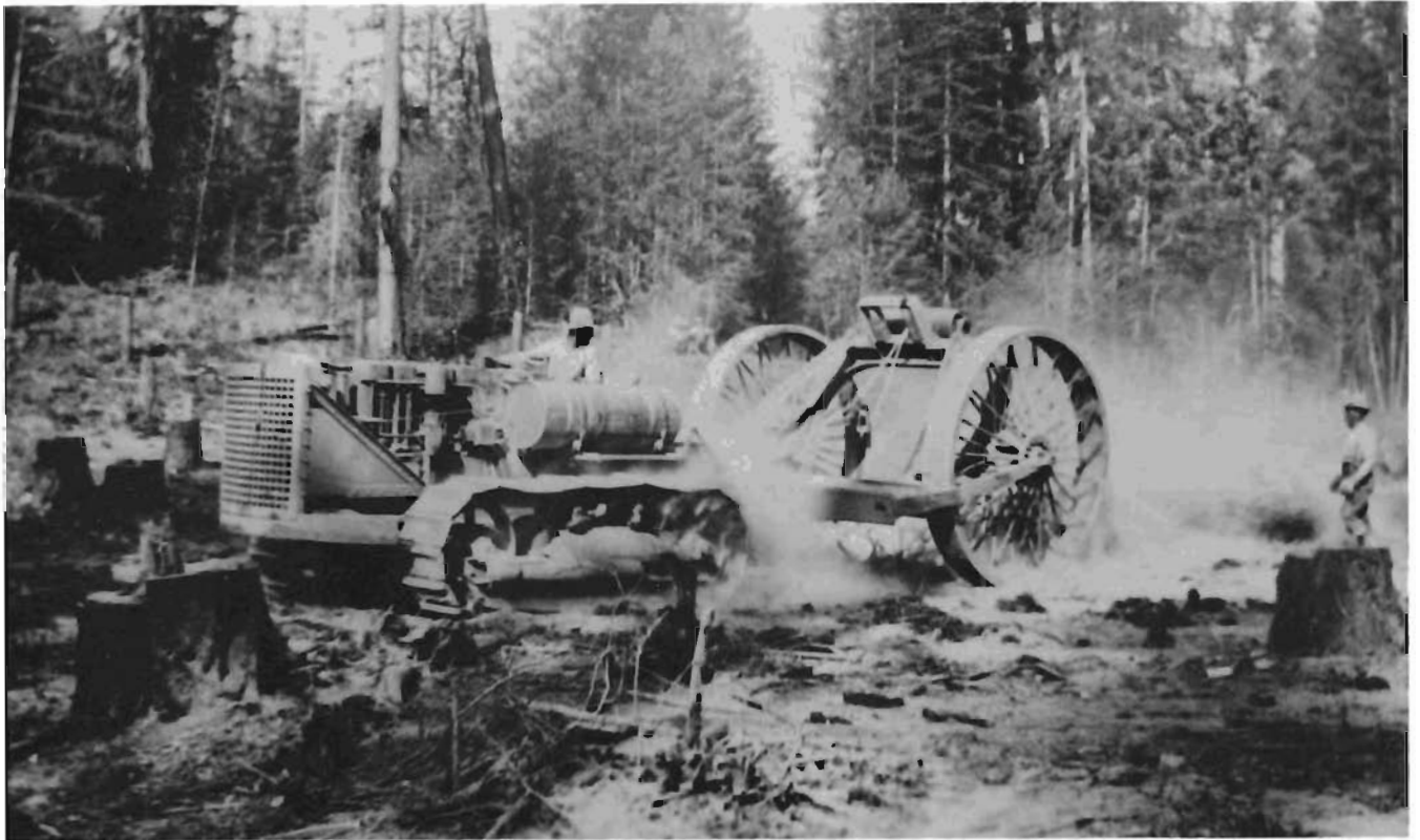
E. R. Aston Caterpillar tractor and hydraulic log lift high wheels being demonstrated at the first company picnic on August 21, 1927 near Camp 6 located on the "B" line.
