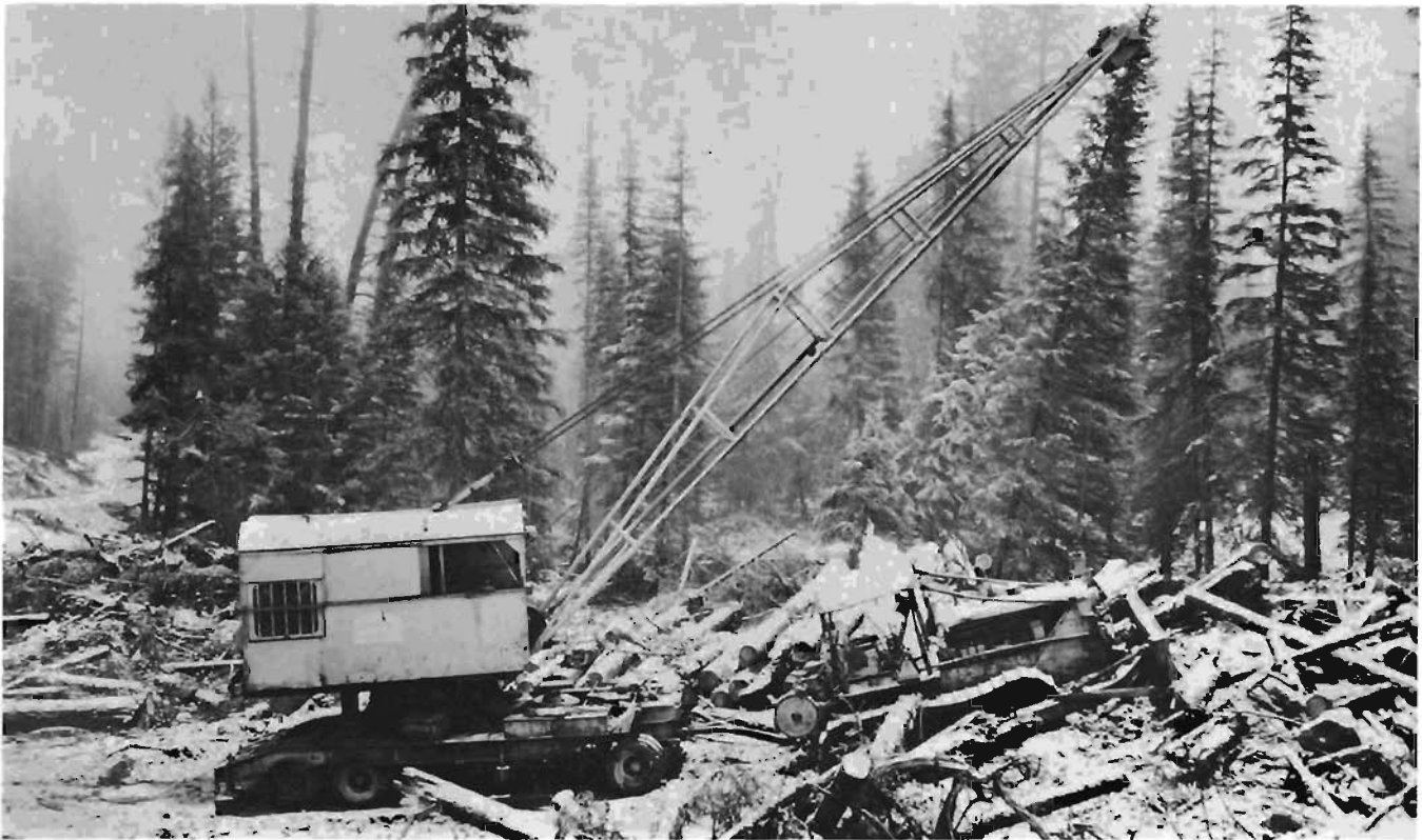
Side view of the Biles-Coleman Lumber Company "Buncher" being used for log loading along the Moses Meadows road during October 1965.
