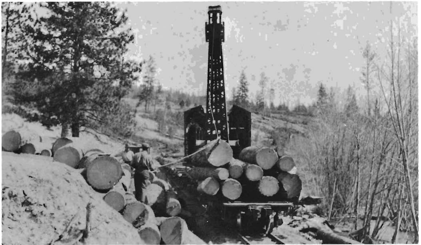
E. R. Aston Biles-Coleman Lumber Co. slideback log loader loading logs on log car No. 111 near Disautel, Washington on the "B" line during 1927. (Photo 1 of 4)
