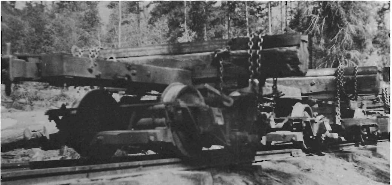
Standard two bunk short log car used on the Omak Mountain line in 1924.
