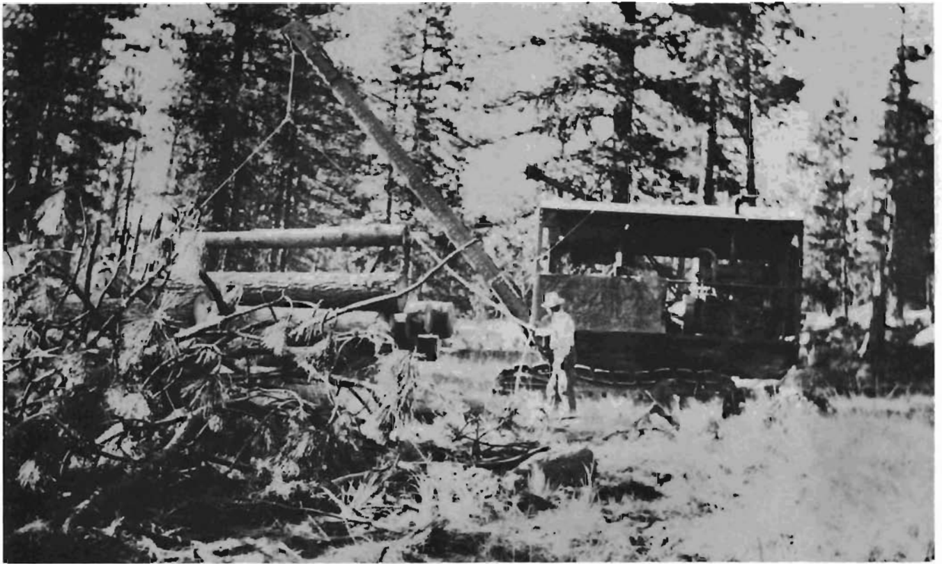
The Biles-Coleman "Buncher" being used to stack logs near the village of Disautel, Washington in September of 1935. E. Fulford
