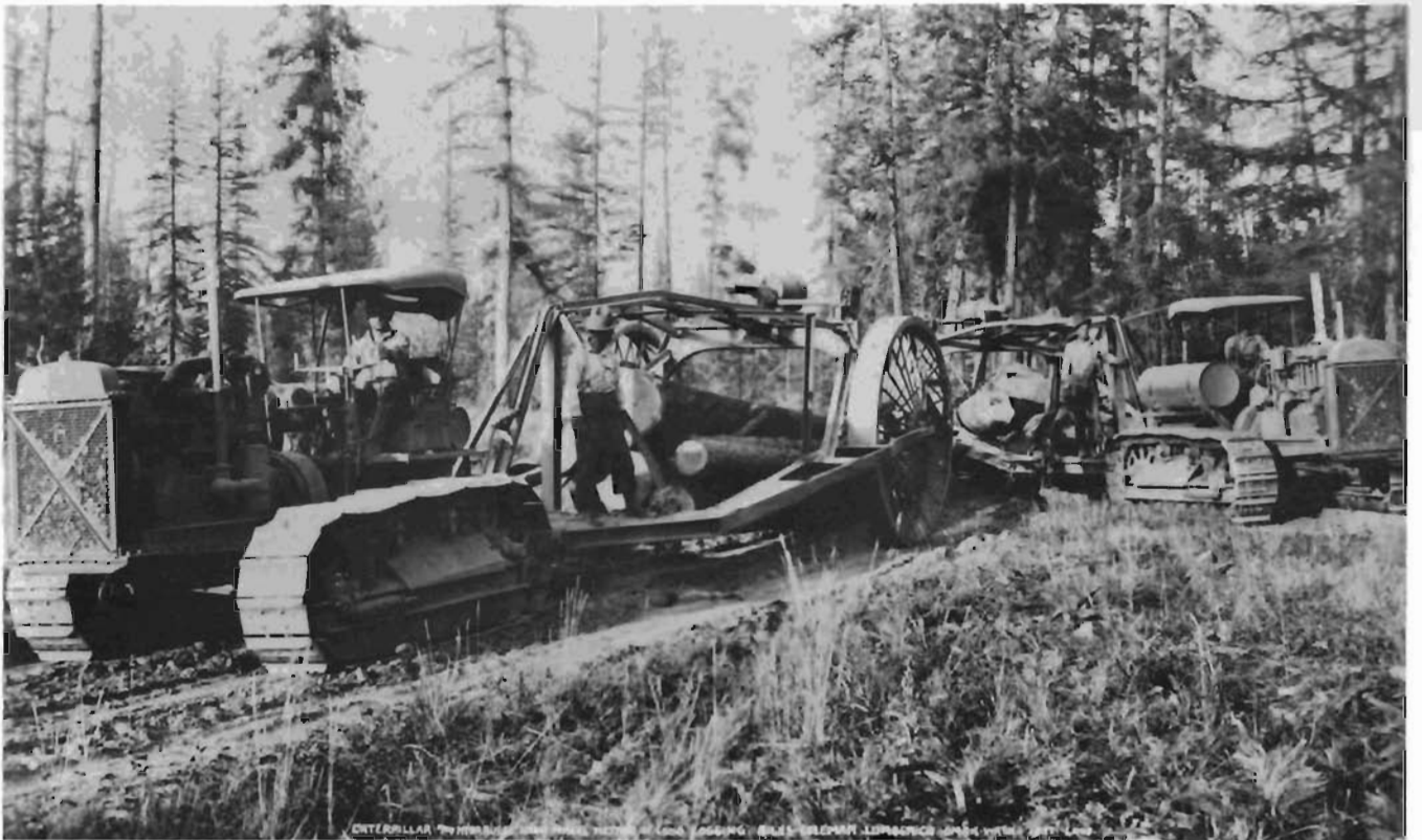
Ladd Photo from E. Aston Caterpillar tractors and hydraulic log lift high wheels being used by Biles-Coleman in 1927 to yard logs to track side.
