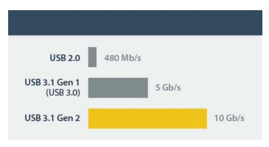
USB 3.1 Gen 2 gives you greater bandwidth and speed with file transfer rates of up to 10 Gbps – twice the speed of USB 3.0 (USB 3.1 Gen 1) technology. It lets you leverage the high performance of the latest SSDs and hard drives, while alleviating bottlenecks in your data transfer.
