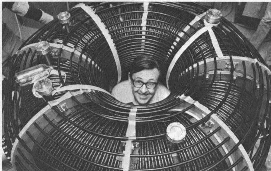
All wrapped up in his work, Roy W. Gould, professor of applied physics, gets the feel of a newly-constructed device, the tokamak, to be used for experiments concerning heating mechanisms in plasmas — work with applications for the production of energy through nuclear fusion. Coils of the tokamak are wound around a stainless steel vacuum chamber where the plasma heating takes place. These coils create the magnetic fields necessary to produce and confine the plasma.
