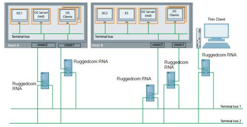
The following RNA devices, also known as redboxes, are recommended for use of the redundant terminal bus with ESXi:
