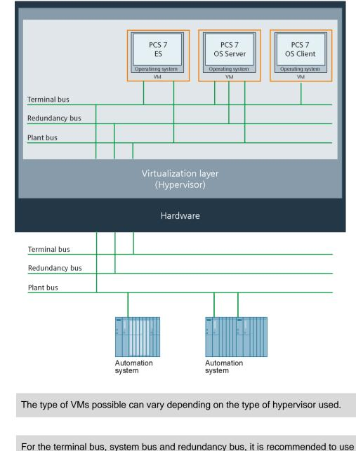
**Note** For the terminal bus, system bus and redundancy bus, it is recommended to use a dedicated network adapter on the host. To connect the ES to the fieldbus (PROFINET), a dedicated network adapter must be used for commissioning and diagnostics.
