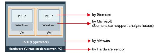
**Note** When using SIMATIC Virtualization as a Service (see chapter <u>3.4</u>) you not only get preinstalled and preconfigured ESXi servers including SIMATIC PCS 7 installations in the form of VMs, you also get the service for these complete systems from a single source.
