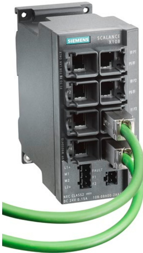
Figure 5-2 Plugging in the IE FC RJ45 Plug 180
