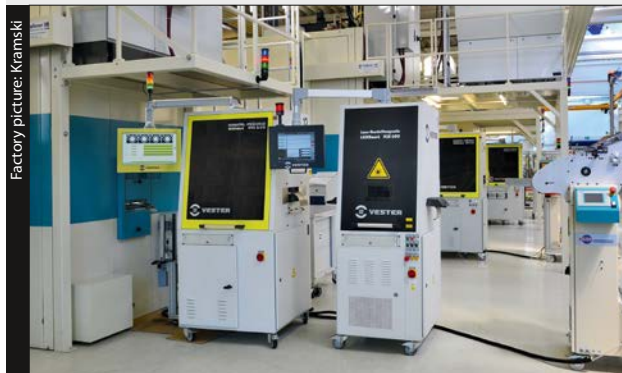
Test cell VIDEOcheck VVC 610 for stampings and LASERmark VLM 600
