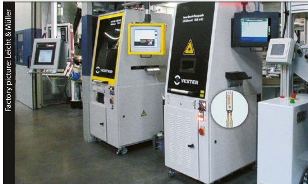
Stamping line with VIDEOcheck VVC 610 and LASERmark VLM 600 : Laser marking of continuously manufactured stampings
