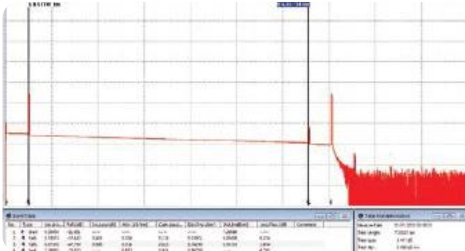
TraceViewer with expanded trace view highlighting the benefit of Launch Cables to examine Near & Far end connectors.
