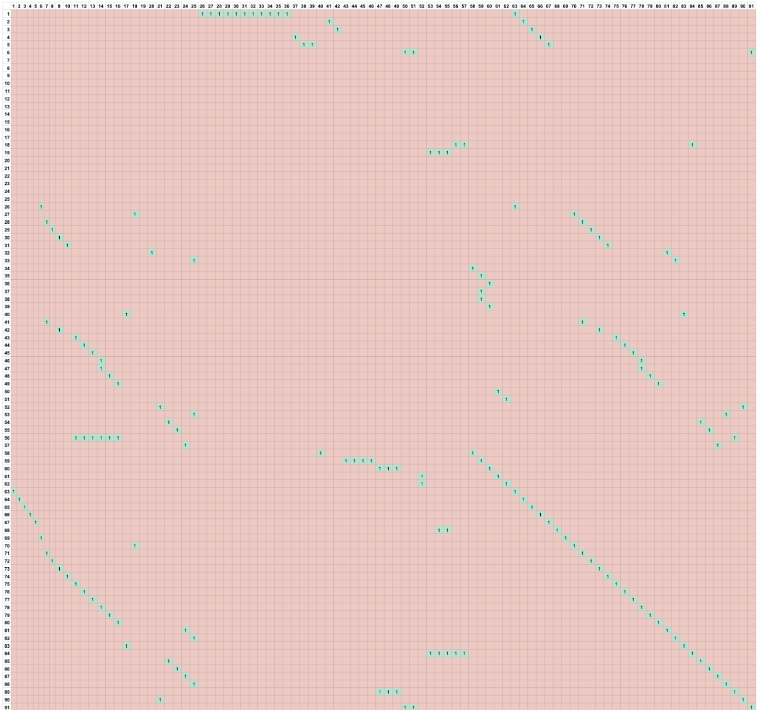
Figure 23 Heterofunctional adjacency matrix The heterofunctional adjacency matrix is a representation of function to form. The heterofunctional adjacency matrix tells us more information about the system than the traditional adjacency matrix because it shows how the formal element of the entire system is connected with each other in a
