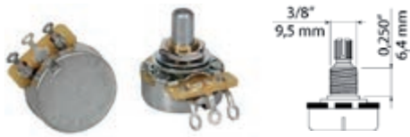
1000K audio potentiometer, solid shaft, short bushing .250", 3/8" diameter, pickguard mount 31721 CTS1MEG-A58
