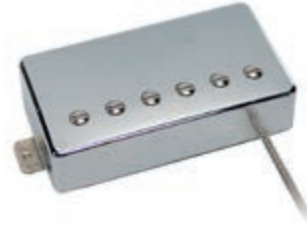
Vintage humbucker, Alnico 5 bar, braided shield wiring, waxed enamel wire, 8.8K bridge
