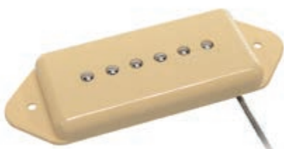
Vintage single coil, Alnico 5 bar, braided shield wiring, waxed enamel wire, 8.0K neck
