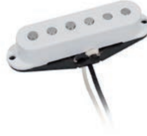
Vintage single coil, Alnico 5 rods, black fiber bobbin, waxed enamel wire
