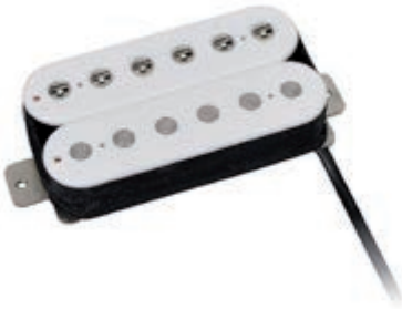
Power Rock humbucker, Alnico 5 bar, 4 conductors, waxed formvar wire, 9.6K neck
