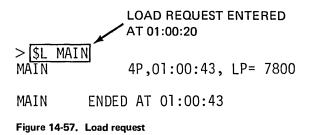
The amount of time elapsed, from the time the ENTER key is pressed to enter the \$L MAIN command to the time the load message is returned, is 23 seconds by stopwatch. The majority of this time was taken in looking up the data set and overlay program locations for the control blocks in the program header.
