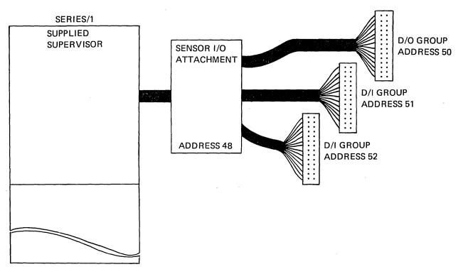
Figure 13-6. Sensor device connections
