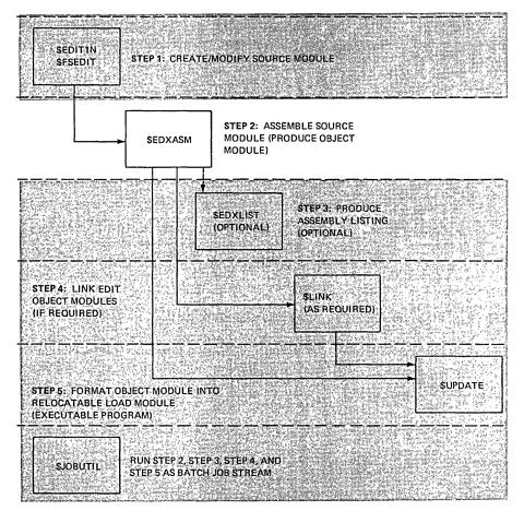
Figure 16-30. Step 2: Assemble source module
