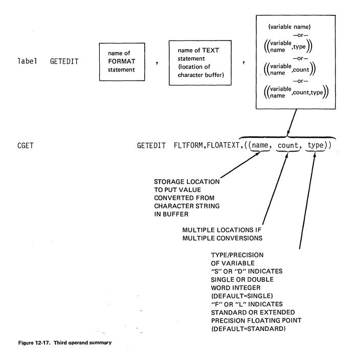
If arithmetic variables are being converted, the data type specified must agree with the data conversion specification in the FORMAT statement (F or L in GETEDIT must have either F or E in FORMAT statement, and S or D in GETEDIT corresponds with I in FORMAT statement).
