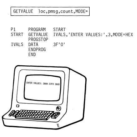
Forms control operands (SKIP=, LINE=, and SPACES=) serve the same purpose and are used the same way with PRINTNUM and GETVALUE as for PRINTEXT and READTEXT. See the reading assignment for how to use PRINTNUM and GETVALUE with double precision integers, standard and extended precision floating point values, and the external data formatting option.
