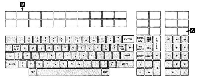
Assuming a standard 4978 keyboard is installed, the \$4978CS0 control store supports the keyboard shown in Figure 14-24. (The unshaded keys are those that will produce hardware interrupts.)
