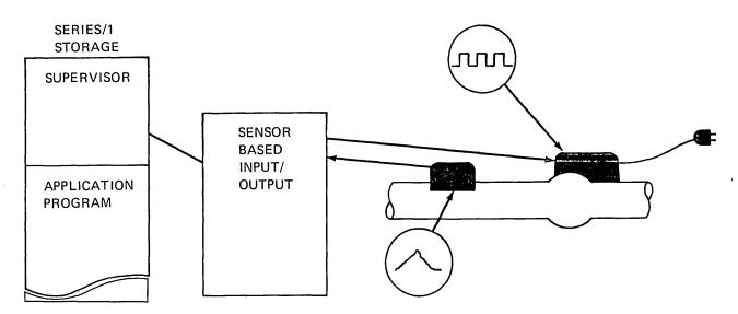
Figure 13-3. Sensor based I/O flow monitoring
