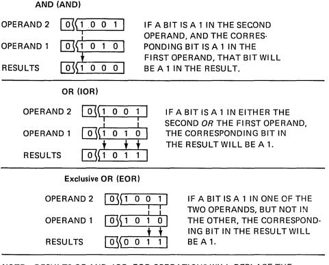
NOTE: RESULTS OF AND, IOR, EOR OPERATIONS WILL REPLACE THE CONTENTS OF OPERAND 1, OR WILL BE PLACED IN THE LOCATION SPECIFIED IN THE RESULTS= OPERAND, IF IT IS CODED.
