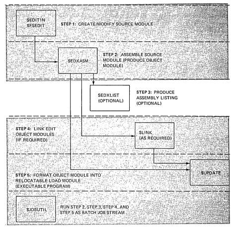
Figure 16-33. Step 3: Produce assembly listing
