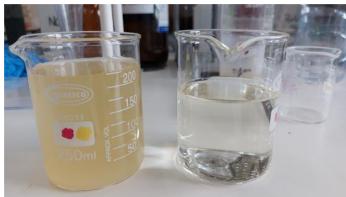
Figure 1 - Slaughterhouse effluent before and after application of the chemical precipitation technique
