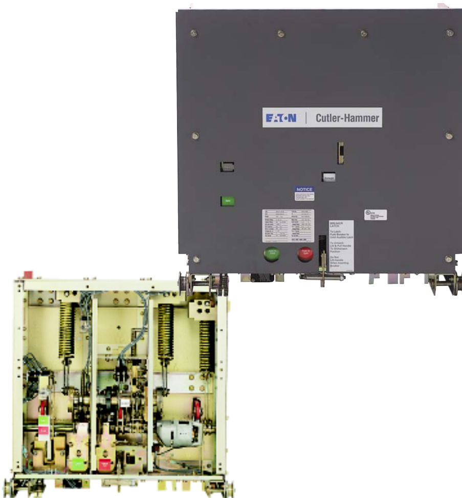
Stored energy mechanism is conveniently located behind the removable front panel. The front mounting of the mechanism provides two dead front shields between the operator and high voltage when the circuit breaker is energized.
