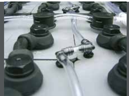
"Z-version": Acid circulation version, cells with acid circulation. Every element contains a little tube in which the charger pumps a little quantity of air which makes the electrolyte circulate from the beginning of the charge (cf diagram)
