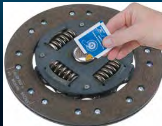
Apply lubricant sparingly and remove excess
