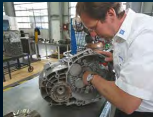
Clean the bellhousing and clutch actuation system first
