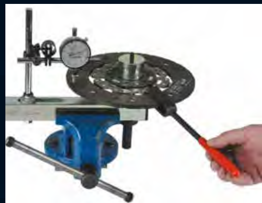
Check the driven plate for lateral runout
