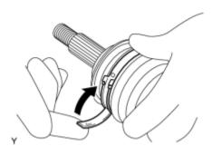
(a) Install the front No. 2 axle outboard joint boot clamp onto the outboard joint boot and temporarily fold back the lever.
