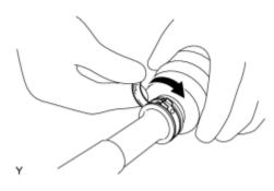
(a) Install the front axle outboard joint boot clamp onto the outboard joint boot and temporarily fold back the lever.
