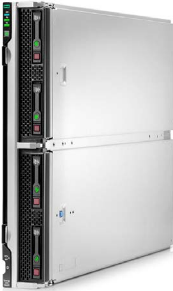
Figure 2. HPE Synergy 660 Gen10 Compute
