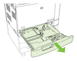
NOTE: Do not open the input tray while it is in use. Doing so can cause jams in the product.
