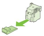
6. Hold the new cartridges so that the arrows on the cartridges align with the arrows on the staple cartridge unit and insert them into the unit.
