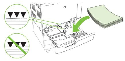
Slide the tray into the product. The control panel shows the tray type and size configuration. To specify specific custom dimensions, or if the type is not correct, touch Modify when the control panel prompts to change the size or type.
