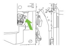
3. Lift up on the small lever at the back of the staple cartridge.
