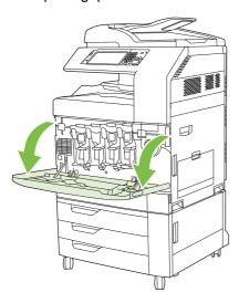
Grasp the handle of the used print cartridge and pull out to remove. 2.
