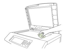
△ CAUTION: Do not pour or spray liquids directly onto the scanner glass. Do not press hard on the glass surface. (You could break the glass).
