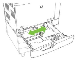
Adjust the paper length guide by squeezing the adjustment latch and sliding the guide to the size of the paper being used.
