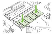
NOTE: If you have difficulty inserting the DIMM, make sure the notch on the bottom of the DIMM is aligned with the bar in the slot. If the DIMM still does not go in, make sure you are using the correct type of DIMM.
