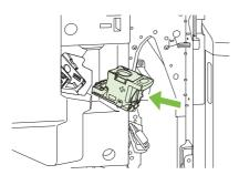
**4.** Push the staple cartridge unit into the stapler unit until it clicks into position.
