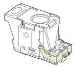
**6.** Reinsert the staple cartridge into the finishing device, and push down on the green handle until it snaps into place.
