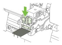
6. Pull the staple cartridge unit forward, and swing it downward to the original position. Push in on the handle to lock it into position.
