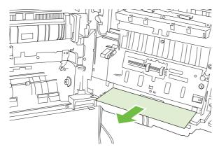
3. If paper has entered the internal paper path, lift the green handle on the transfer-access panel and open the panel.
