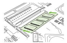
9. Push down on the DIMM until both latches engage the DIMM.
