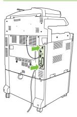
11. Reconnect the power cable and interface cables, and turn the product on.
