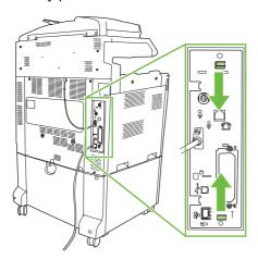
**5.** Gently pull on the black tabs to pull the formatter board from the product. Place the formatter board on a clean, flat, grounded surface.
