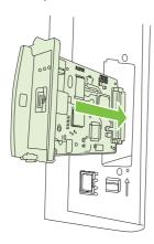
5. Insert and tighten the retaining screws that came with the print server card.
