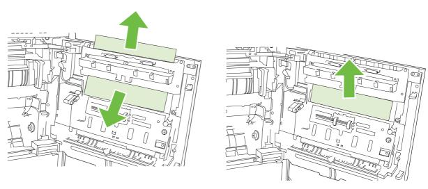
4. Lift the paper-feed cover on the inside of the right door. If jammed paper is present, gently pull the paper straight out to remove it.
