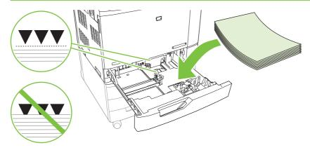
NOTE: For best performance, fill the tray completely without splitting the ream of paper. Splitting the ream can cause a multifeed problem. The capacity of the paper tray can vary. For example, if you are using 75 g/m² (20 lb) paper, the tray holds a full ream of 500 sheets. If the media is heavier, the tray will not hold a full ream. Do not overfill the tray.
