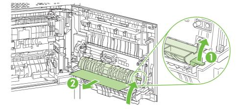
5. Lift the green handle on the transfer-assembly and open the panel.
