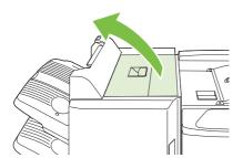
2. Remove jammed paper from the output bin or from the inside of the finishing device.
