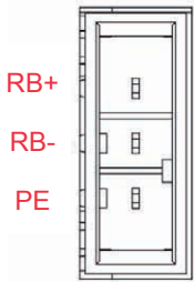
Front view of connector on controller side
