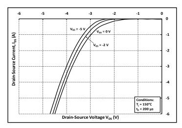
Figure 10. Body Diode Characteristic at 150°C
