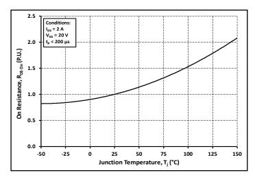
Figure 4. Normalized On-Resistance vs. Temperature
