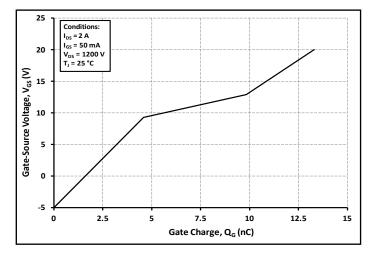
Figure 12. Gate Charge Characteristics
