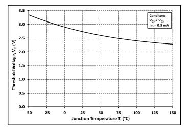
Figure 11. Threshold Voltage vs Temperature
