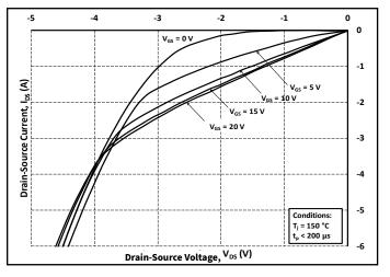
Figure 15. 3rd Quadrant Characteristic at 150°C
