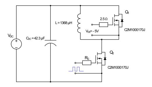
Figure 29. Clamped Inductive Switching Waveform Test Circuit
