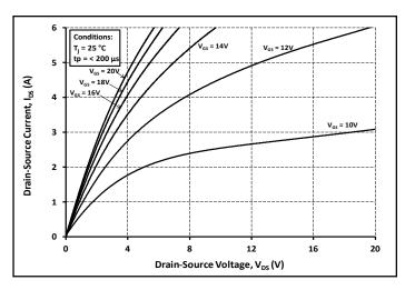
Figure 2. Output Characteristics T<sub>J</sub> = 25°C
