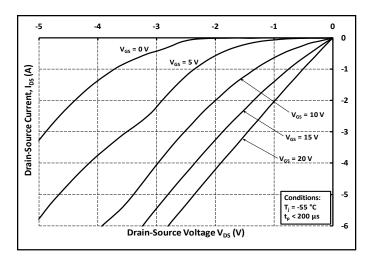
Figure 13. 3rd Quadrant Characteristic at -55°C
