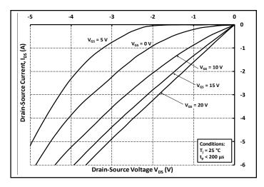
Figure 14. 3rd Quadrant Characteristic at 25°C
