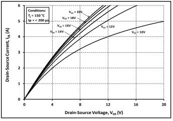
Figure 3. Output Characteristics T<sub>J</sub> = 150°C
