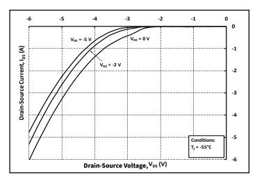
Figure 8. Body Diode Characteristic at -55°C
