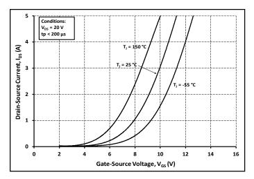
Figure 7. Transfer Characteristic for
