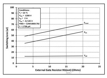
Figure 25. Clamped Inductive Switching Energy vs. R<sub>G(ext)</sub>
