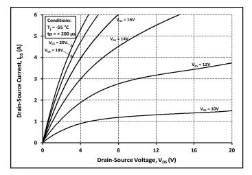
Figure 1. Output Characteristics  $T_J = -55^{\circ}C$
