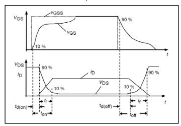
Figure 28. Switching Times Definition
