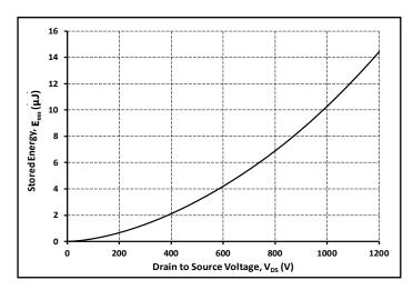
Figure 16. Output Capacitor Stored Energy
