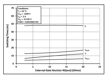
Figure 27. Switching Times vs. R<sub>G(ext)</sub>
