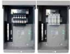
MNPV6 with 150VDC breakers and with 600VDC fuses
