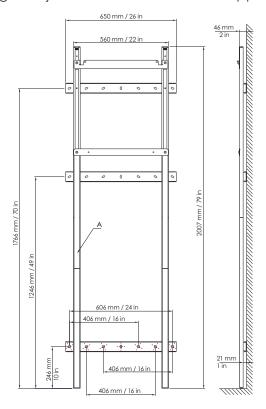
Height-Adjustable Wall Mount Floor Support for 86" Size
