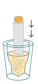
Magnetic beads mix with sample, binding to target
