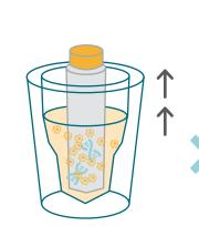
Magnetic rod is lowered into the solution; magnetic beads and target collect at the bottom of the tip comb
