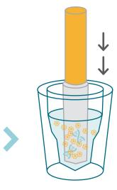
Beads are then released by moving the magnetic rods out of the tip comb; tip comb also facilitates the mixing of reagents with the beads as the magnetic head moves up and down
