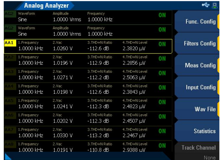
Figure 4. The U8903B's GUI, showing 8 analyzer channel measurements.
