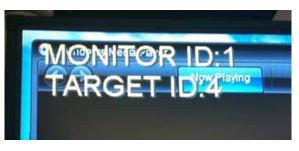
7. Use the TileMatrix feature to setup the 3x3 Video Wall. The Tilematrix feature of the NEC Display allows for one image to be expanded and displayed over a 2x3 Video Wall Setup.\* This is accessed through the OSD (On-Screen Display) Controls under the "MULTI-DSP"
