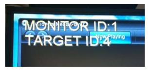
7. Use the TileMatrix feature to setup the 2x2 Video Wall. The Tilematrix feature of the NEC Display allows for one image to be expanded and displayed over a 2x2 Video Wall Setup.\* This is accessed through the OSD (On-Screen Display) Controls under the "MULTI-DSP"
