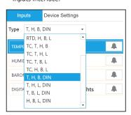
The SS-002-0 offers a configurable choice of one external thermocouple, RTD, or DIN (contact closure).
