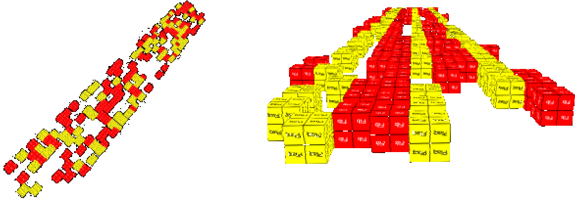
Figure 2: the left screenshot shows the initial state of the system, which is a set of agents located at random. The right image shows the formed a linear structure after 100 steps of simulation.
