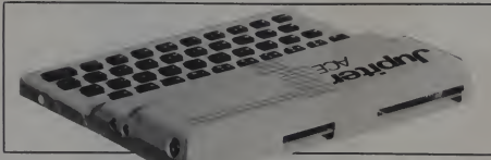
The rear view reveals the Z80 pinout and an edge card connector.
