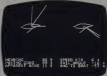
Photo 5. Vector diagram of the beam reach. Notice that the total force vector is smaller than during the windward sailing but the boat is moving faster. This is because the forward component is larger for a reaching situation, and the leeway is less.
