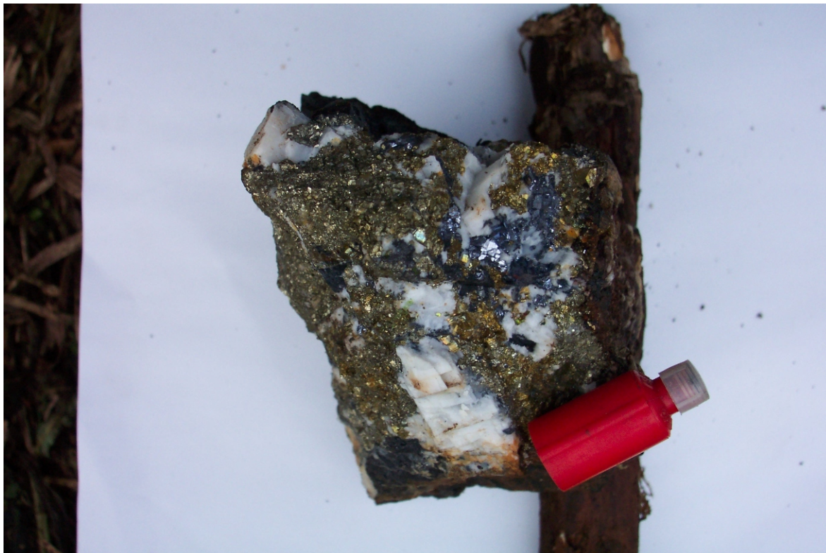
Figure 5b: Massive carbonate sulphide vein found in Keiths Creek. Sample contains approximately 50% calcite, 25% pyrite, 15% sphalerite, 10% galena and trace chalcopyrite (visual estimate).
