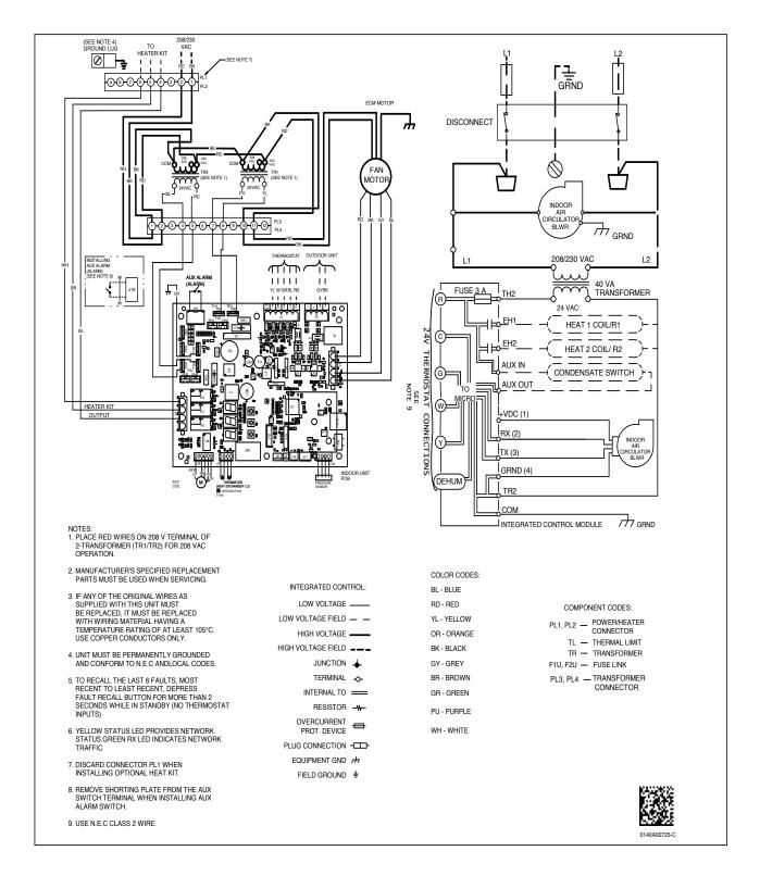
Wiring is subject to change. Always refer to the wiring diagram on the unit for the most up-to-date wiring.
