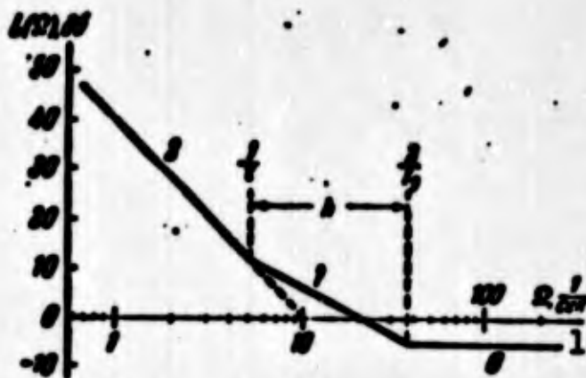
Fig. 150. Logarithmic amplitude characteristic and gain-phase characteristic for Problem 259. 1) sec.
