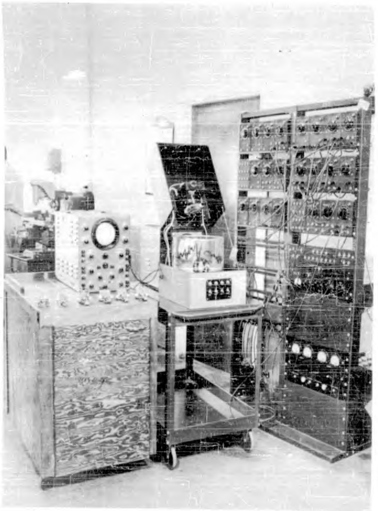
FIGURE 82. PHOTOGRAPH SHOWING ANALOG COMPUTER AND FUNCTION GENERATOR
