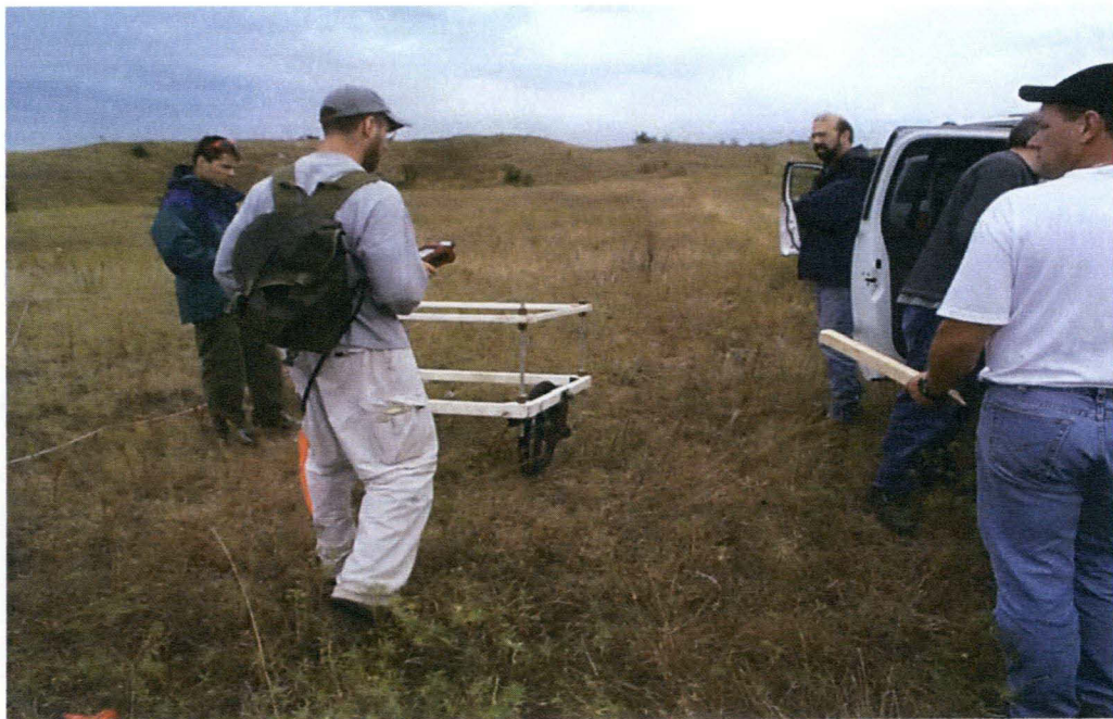
Figure 6. Well Location Proofing Using EM-61
