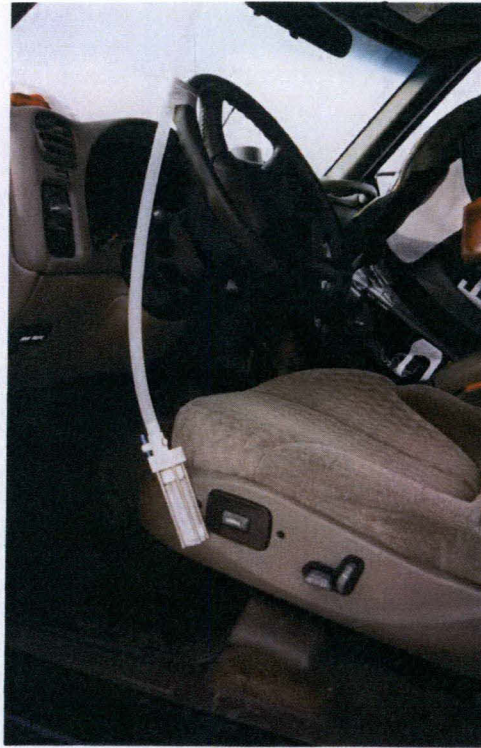
Figure 25. Double Needle Device for Sampling VOC's
