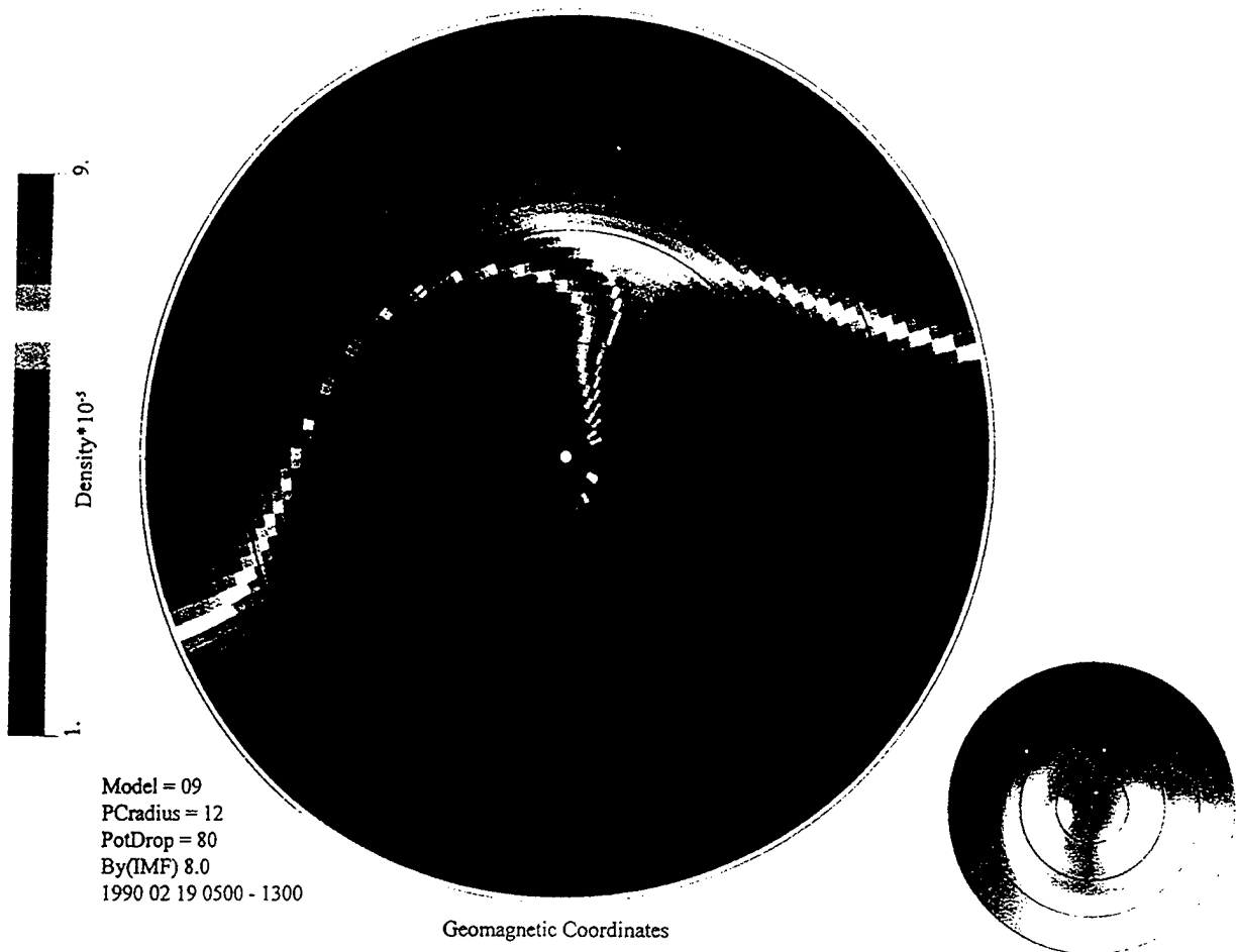
Plate 1. Polar plot of the NmF2 (peak F region density) of the high-latitude ionosphere at 1300 UT. This density plot corresponds to the initial values used in the simulations of sections 3.1, 3.2, 3.4, and 4. The values in this plot were obtained by running the model for 8 hours and using steady state inputs. We include in the lower right corner the black and white version of this plot in a format that will be shown in subsequent plots. The black dots correspond to the locations of the Sondrestrom and Qaanaaq stations, and the white dot indicates the location of the European Incoherent Scatter station. The latitudinal circles are in steps of 10^\circ .
