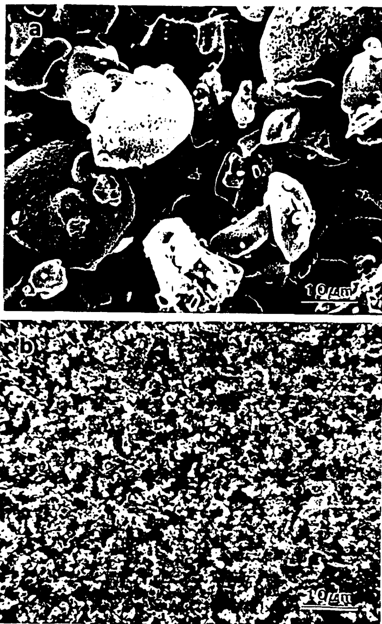
Fig. 9. (a) SEM micrograph of \text{MgSiO}_3 powder calcined at 900\text{ }^\circ\text{C} for 2 h (powder A). (b) The same powder after 5 h of attrition milling (powder B).
