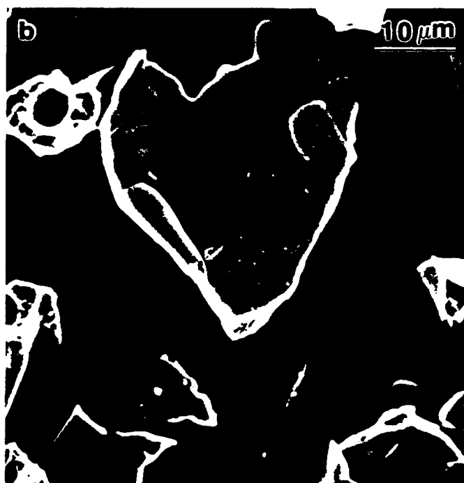
Fig. 6. SEM micrographs of \text{Sr}_2\text{SiO}_4 powder derived from a gel containing 90% resin calcined at (a) 800°C for 1 h (the individual crystallites have sintered together into highly porous agglomerates), and (b) 1400°C for 1 h (the agglomerates have fully sintered).
