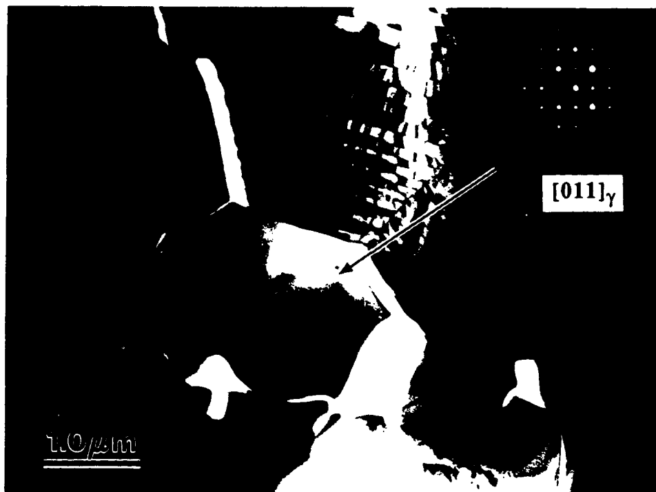
Fig. 13. Transformed \gamma grain retained in \beta grains. Large cracks generated during the \beta \rightarrow \gamma transformation (from single-phase \text{Ca}_2\text{SiO}_4 sample sintered at 1400^\circ\text{C} for 3 h).
