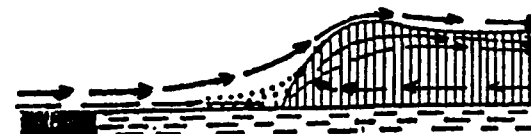
Figure 2-57c. Maximum Compacting of the Marine Boundary Layer. At this instant, the surface winds inside the marine boundary layer shown onshore direction. The marine layer surface flow may take several hours to reach the coast. Momentum accelerates wind speed with time.
