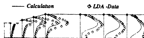
Figure 1 Distribution of the turbulent kinetic energy. Comparison of LDA-measurement with calculation (k-ε)
