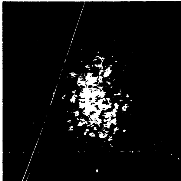
Figure 1. Speckle interferometry, a technology developed during the past 20 years, allows astronomers to overcome the distorting effects of the earth's atmosphere by photographing celestial objects at very short exposure times. A speckle image is a kind of multiple exposure, with each individual speckle containing a complete representation of the object. The speckle image of a star on the left was obtained at the 4-m telescope on Kitt Peak using an electronic camera with an exposure time of 1/30 second. The field of view is just under 3 sec of arc. In a four-second exposure of the same star (right), the fine speckle detail has been blurred by the rapidly changing atmosphere. (All photographs are by the author.)
