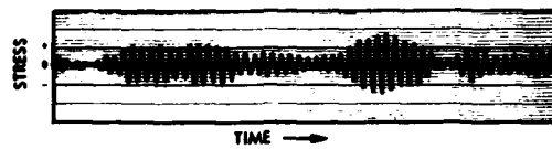
Figure 6. Stress-Time Response Profile of Single-Degree-of-Freedom System
