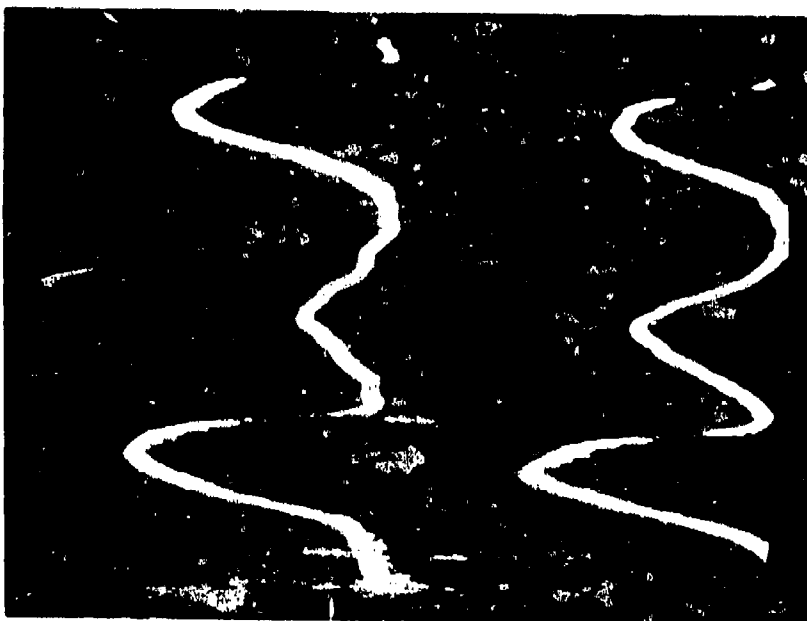
FIGURE 3. TV MONITOR DISPLAY OF A DATA FRAME. The time scale runs downward and spans 50 ns; signal deflections are to left. Unpolarized receiver trace is on right, cross polarized on left. Signal deflections, in sequence, are the reference pulse, the aerosol backscatter pulse, and the diffuse target pulse. Frame is from trial 14.
