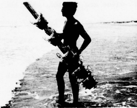
Figure 20. Photo of simultaneous water sampler ready for sampling 5 positions above the bed. Total weight with 4 empty bottles is 10.5 kg.
