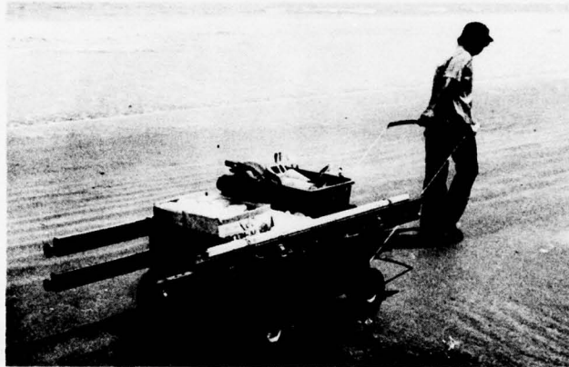
Figure 23. Custom beach cart designed by D. Domeracki used to haul samples and equipment 2 miles down the beach for ferrying to a nearby lab. Brackets at the sides hold sampler poles, profile rods, range markers. Along the open beach, sand is hard-packed, making it relatively easy for 1 person to haul the 200 + kg weight. This is not the case, however, near the inlet where the sand is almost thixotropic.
