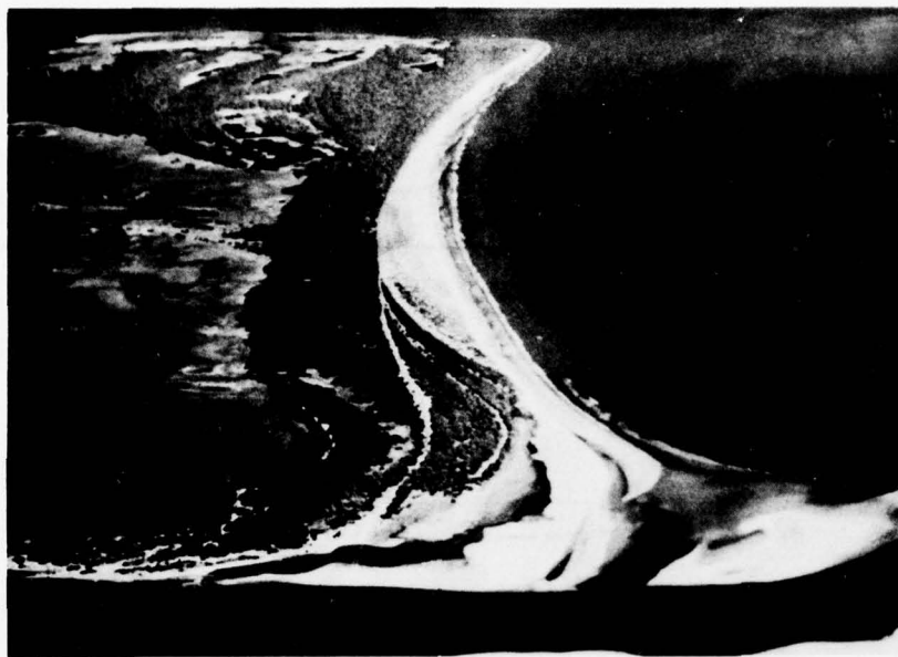
Figure 13. Oblique IR aerial photo of Bulls Island, looking northeast. Net sediment transport is southeast at 1.3 \times 10^5 \text{ m}^3/\text{yr} . (Kana, 1977).
