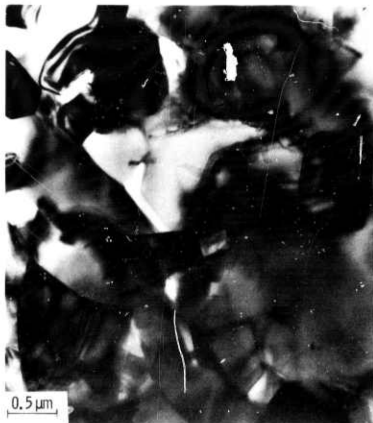
Figure 5.28 — Typical pores in hot pressed silicon nitride. The sharp transition in contrast at the edge of a pore indicates that it was not due to thinning effects (800 kV, 15^{\circ} thinning)
