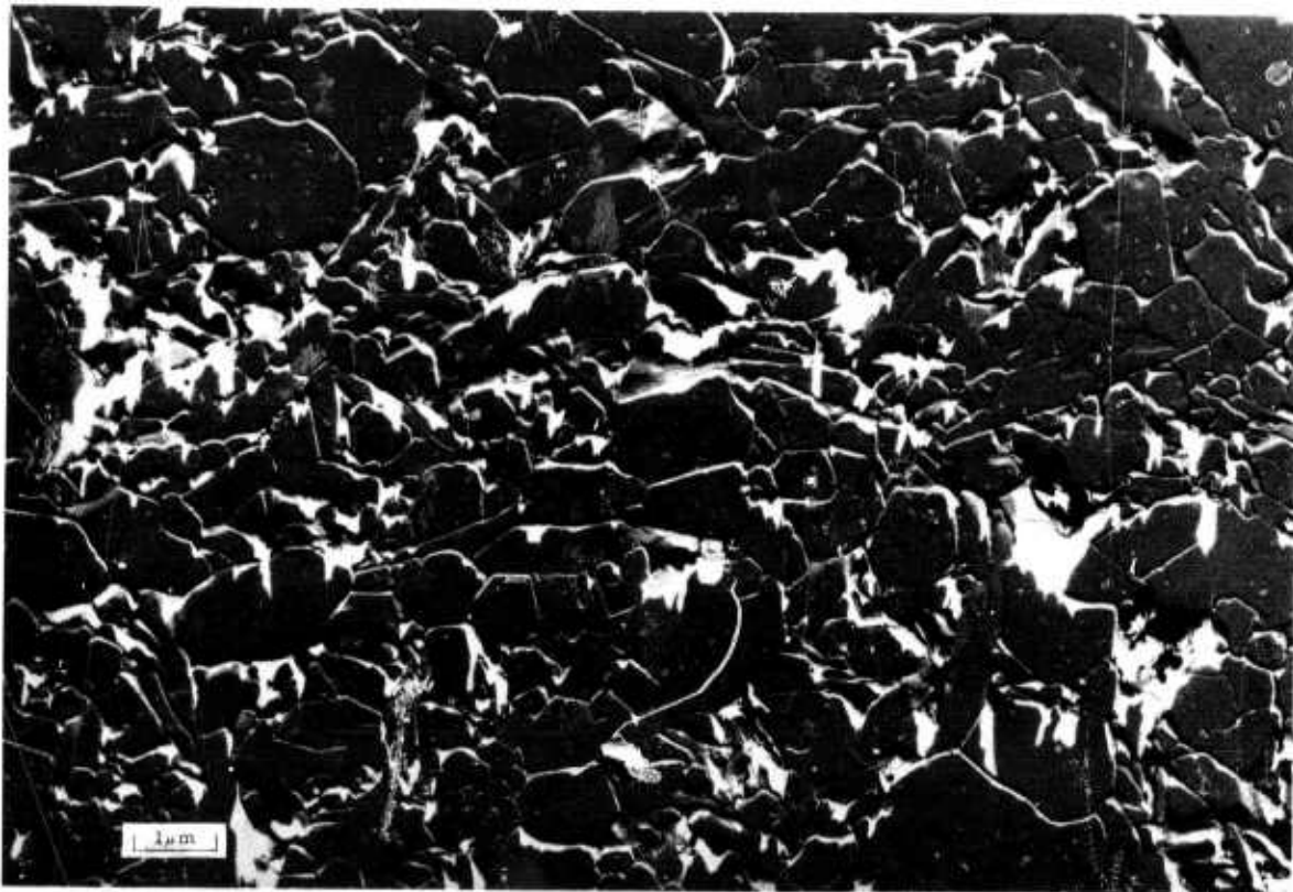
Figure 3.9 — Electron Micrograph, 18,800X of Etched Lucas Hot Pressed Silicon Nitride
