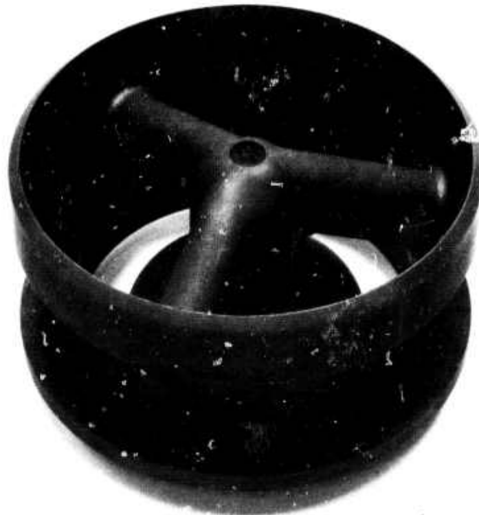
Figure 3.44 — Nose Cone as Molded
