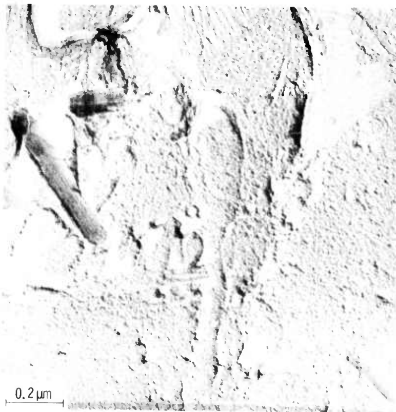
Figure 5.20 -- High magnification detail of an over etched surface of hot pressed \text{Si}_3\text{N}_4 . Two stage carbon replica
